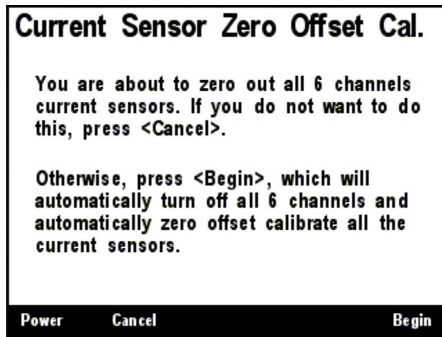
Figure 53 – DCR100 Current Sensor Zero Offset Calibration Screen
