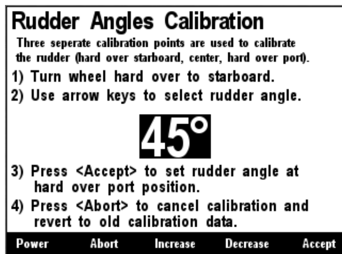
Figure 147 – RAA100 Starboard Rudder Angle Calibration
